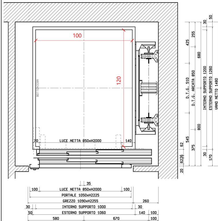
SCHEMA PIANTA PIATTAFORMA ELEVATRICE - Scala 1:10
