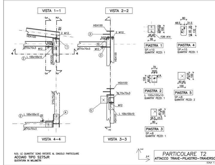
**PARTICOLARE T2 ATTACCO TRAVE-PILASTRO-TRAVERSO**
